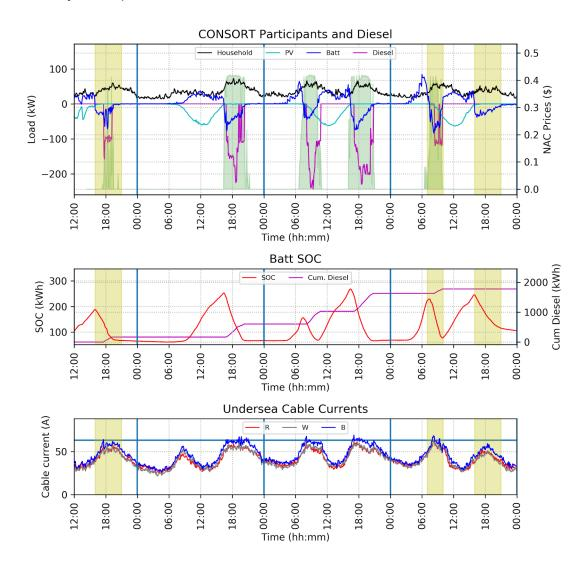
Queen's Birthday long weekend trial. Top: aggregate participant loads, diesel load; negative = generation. Yellow bars are peak TOU tariffs. The pale green filled graph represents non-zero NAC prices. Middle: aggregate battery state of charge, cumulative diesel discharge. Bottom: current in the
