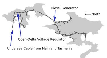
The Bruny Island 11 kV network, which is modelled by the NAC in order to optimally coordinate DER dispatch.
