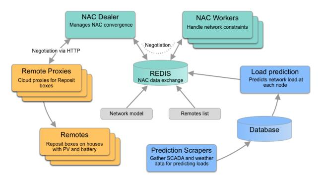
Detailed NAC architecture, as implemented in CONSORT. Different systems are highlighted in different colours: teal for the NAC, orange for the remotes, and blue for the load prediction.
